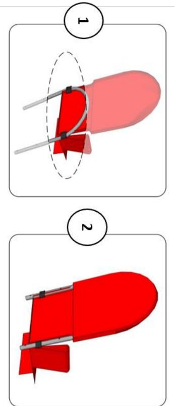
Install the arm rests to the seat base. Insert the armrests through the fabric sleeves. Secure the hook and loop closure.
