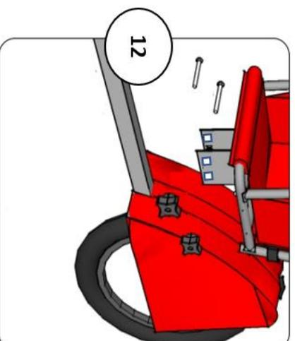
You may also use pliers on the knob to help tighten. Continue tightening until there is little to no movement on the frame.
