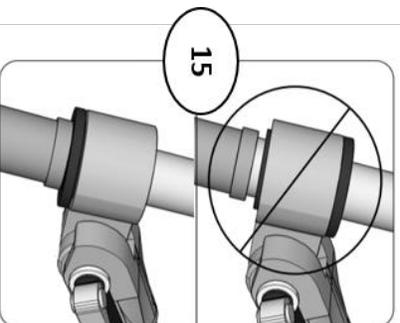
Insert the hitch around the bushing. Drop the receiver onto the hitch, then insert and secure the quick release pin.
