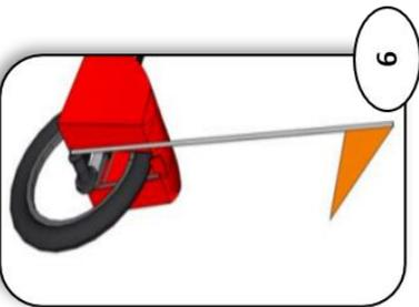
Install the reflector with the bushing included around the frame on top of the back wheel.
