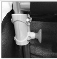
To collapse the trailer, pull out on the red knobs and white elbows simultaneously.
