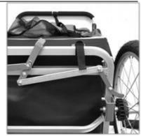
When parking brake is engaged make sure the arm is fully inserted between the teeth of the wheel.
