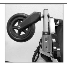
Take the quick release pin and insert it into the back hole of the stroller wheel receiver. Push the wire lock over the pin.
