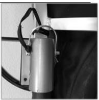
Install the cover using the Velcro straps at the top and elastic loops at the bottom.
