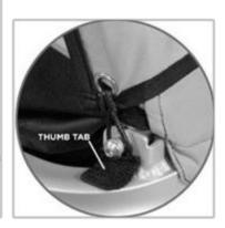
Installing bicycle tow attachment. Ensure spring button engages hole. Install and latch the pin into the second hole.
