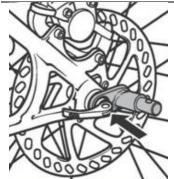
Warning! Ensure the safety loop is secured around the bicycle frame. Wrap the nylon loop around the frame enough times to ensure it does not hang loosely to become entangled in the bicycle wheel or brake. Install the pin and secure the latch.
