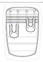
Install the wheels by depressing the rubber button in the center of the wheel, inserting the axle into the frame, then releasing the rubber button.
