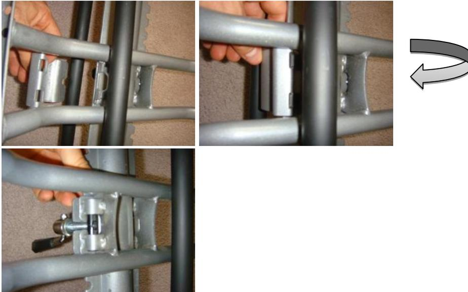
Tighten the quick release into one of the adjusting notches.
