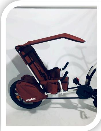
Install the sunshade onto the backrest and its all weather shell. Or store it in the pannier to use later during inclement weather.
