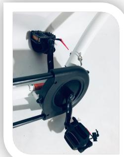
Install the safety flag. Loosen the left axle nut, insert flag, then retighten the axle nut. Install the fender using the hook and loop strap.
