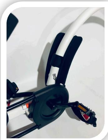
Install the seat onto the frame. Swing the bolts into place then tighten them using the 5mm hex key. 8Nm is the
