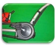
Mark the insertion height of the seat post while it remains in the bicycle. Remove the seat post from the bicycle. Choose the plastic bushing that provides the tightest fit between the hitch and seat post and that can be inserted by hand without tools. Ensure the flange on the bushing is on the bottom side of the hitch.
