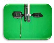
Install the push bar and insert the quick release into the bottom hole. The other two holes can be used to level the iGo on different size bicycles.
